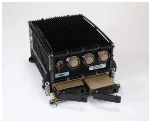
▲ The Phoenix International Phalanx II is SWaP-optimized and provides high performance, high capacity, and secure data storage for unmanned aerial, underwater and surface vehicles and crewed intelligence and surveillance applications.
